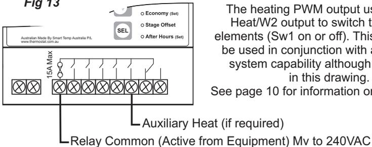
The heating PWM output uses the Aux Heat/W2 output to switch the heating elements (Sw1 on or off). This function can be used in conjunction with a normal A/C system capability although not shown in this drawing.
