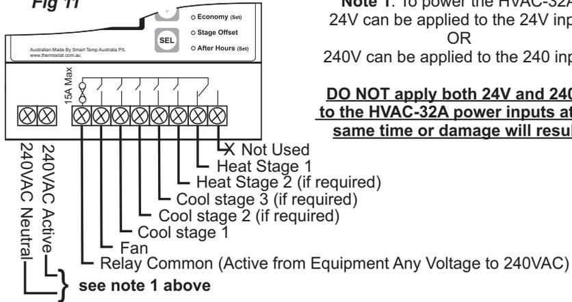
**Note 1:** To power the HVAC-32A 24V can be applied to the 24V input OR 240V can be applied to the 240 input.
