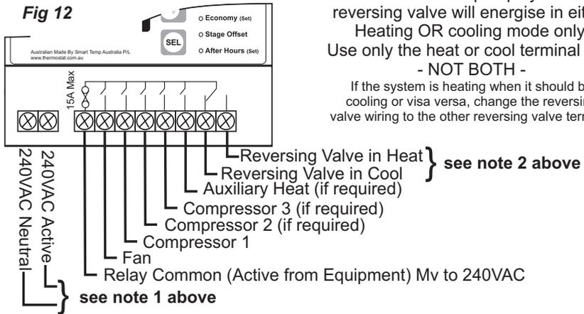
**Note 2:** A heat pump systems reversing valve will energise in either Heating OR cooling mode only. Use only the heat or cool terminal only - NOT BOTH -
